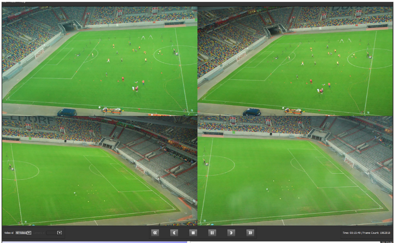
Fig 3. Exemplary still image of the camera setup at one of the four locations. The image shows four camera angles that are subsequently used to provide two panoramic pictures to be used as a stereo pair.
