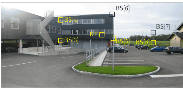
Figure 7. (a) Top view of schematic diagram of the LPM setup at the test site and (b) photograph taken at approximately position x = 0 m, y = -20 m looking in the direction of BS[5]. The true position of the RT is x = -0.327 m, y = 23.575 m, z = 1.588 m and of the MT x = -0.002 m, y = 17.068 m, z = 1.297 m.
